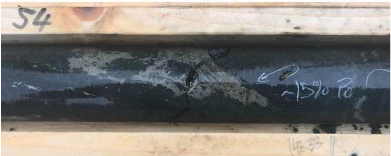
Hole CL-20-09: Coarse sulfide patch at 148.30m in hole CL-20-09 at the equivalent depth of target zone in historic hole 90-70
