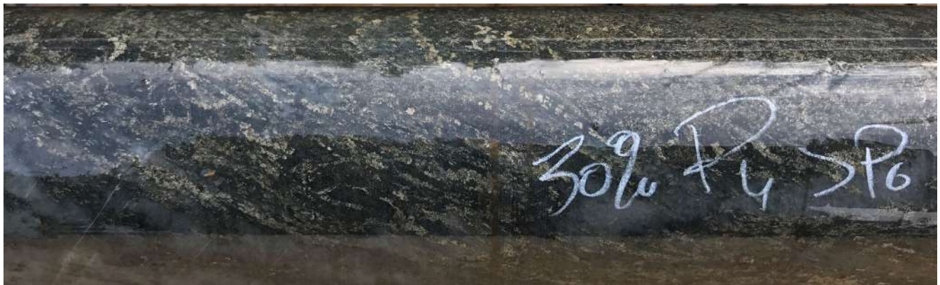
Hole CL-20-08: Intense sulfide replacement and quartz flooding in the target zone of the Bugow Iron Formation
