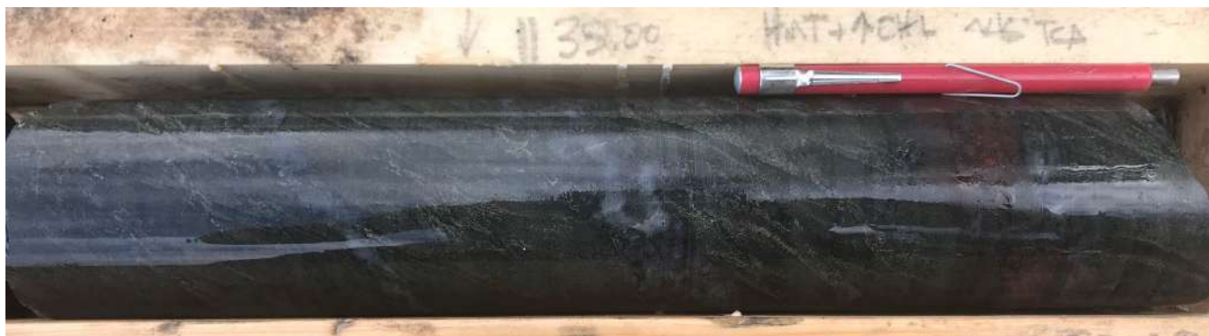
Semi-massive zones of sulfide replacement of the Bugow Iron formation in hole CL-20-01 (approx. depth 35m)
